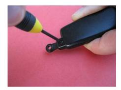
Remote key cases are made of plastic and they are prone to breakage especially around the key ring loop. In most cases the key ring loop is the first to give. Majority of the keyring loops are not exchangeable. Fortunately some loops are made separate to the plastic shell and can be replaced with no problem at all. Just follow simple instructions as below, if your keyring loop attaches to the remote as picture on the left shows.
